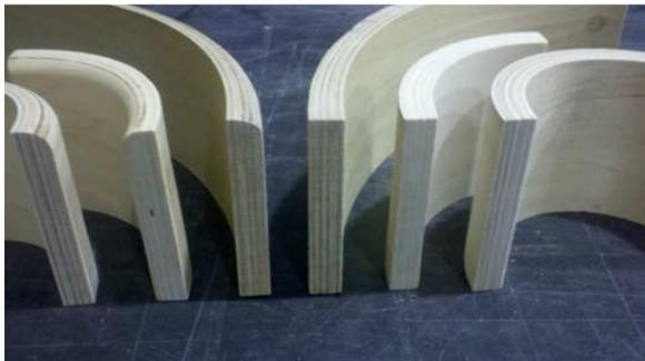
The trim is 5/8" thick with an internal radius to match the Curve panels and a rounded top. Specify height from 2" to 12". 1/4" to 1/2" higher than the base trim provides a nice feature corner. Install with baseboard adhesive, prime & paint. Less work than traditional square corners – no miters to cut.
