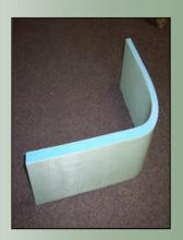
**Thermal Insulation** - Fulcrum Micro-Comb has an R-value of 5, making it comparable to most standard insulating foams. The closed cell structure and high moisture resistance ensure that the thermal insulation is maintained over time – unlike PU foam which degrades with exposure to moisture.
