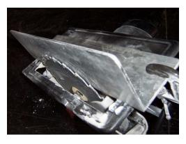
Clamp fence onto standard cut-off saw 1/16" from 0.1" (not 0.080") blade. Set blade depth to 1 5/8".
